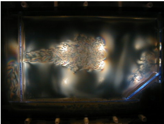
Jet in ambient fluid, V=2\text{cm/s} , 15cm horizontal field of view
