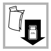
9. Wipe the blank and insert the blank into the cell holder.
