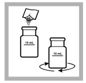
**Prepared Sample:** Add the contents of one Molybdate Reagent Powder Pillow for High Range Silica to the sample cell. Swirl until completely dissolved.
