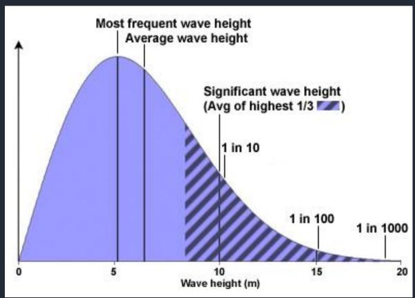
• Significant wave height  $(H_S) = average$  height of the largest 1/3 of waves
