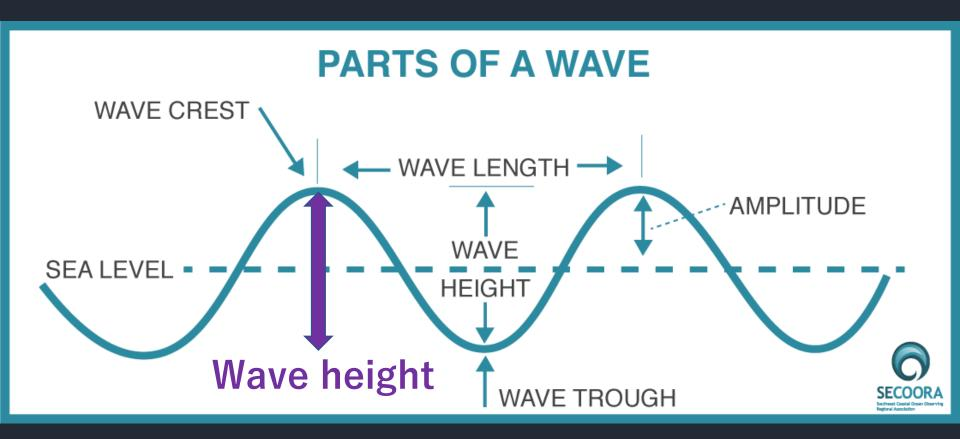
• Significant wave height  $(H_S)$  = average height of the largest 1/3 of waves
