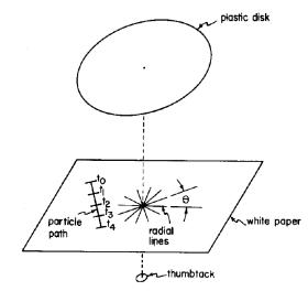
Fig. 1. Exploded view of Coriolis machine.
