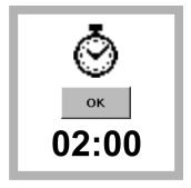
A two-minute reaction period will begin. If the sample was digested using the Acid Persulfate digestion, a ten-minute reaction period is required.
