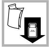
**6.** When the timer expires, wipe the blank and insert it into the cell holder.
