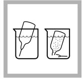
3. Prepared Sample: Fill a PhosVer 3 Phosphate AccuVac Ampul with sample. Keep the tip immersed while the Ampul fills completely.
