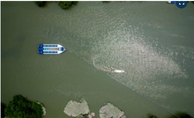
1/2 The Interceptors™ will be placed in strategic locations in rivers to make sure the main plastic flow is intercepted, meanwhile allowing for boats to pass.
